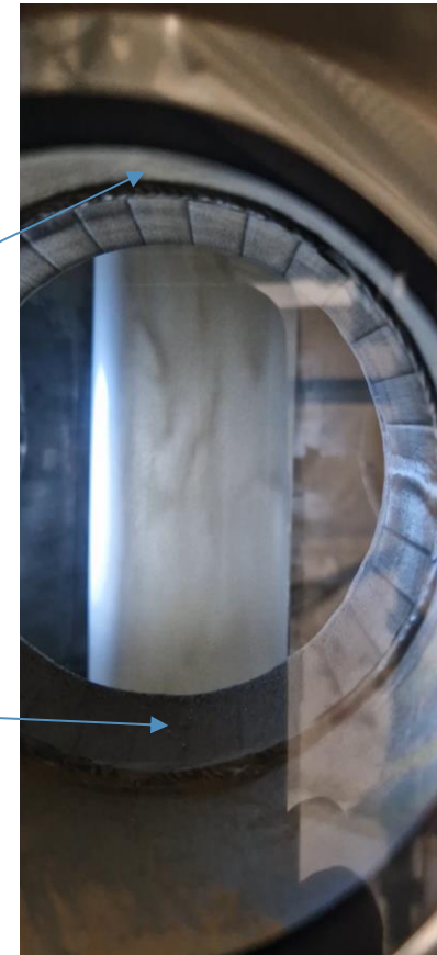
Bed and biomass particles circulated in the standpipe
