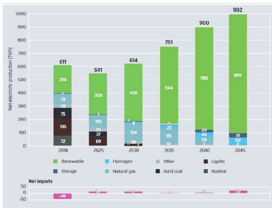
Figure 53: Net electricity and import balance for climate neutrality until 2045 (Graichen et al., 2021)
